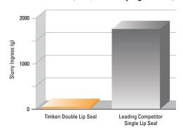
Slurry ingress test results of the optimized Timken Type E seal compared with the single lip seal design of a leading competitor. Seal operating at 250 rpm in a salt and mud slurry mixture for 75 hours.
