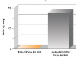
Water ingress test results of the new Timken Type E seal compared with the single lip seal design of a leading competitor. Seal operating at 250 rpm with three gallons of water per minute directed at the shaft-seal interface for four hours.
