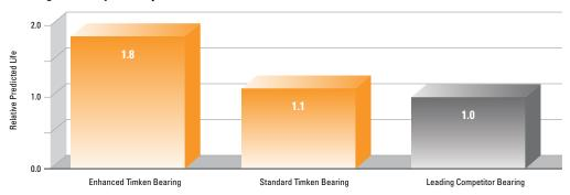
Analytical analysis of the new, optimized Timken bearing compared to a standard Timken bearing (used widely by most Type E suppliers) and a new bearing from a leading industry competitor.
